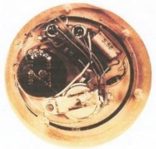
First implanted Elmqvist's pacemaker Weight: 73,4 gr Size: 35 cc
